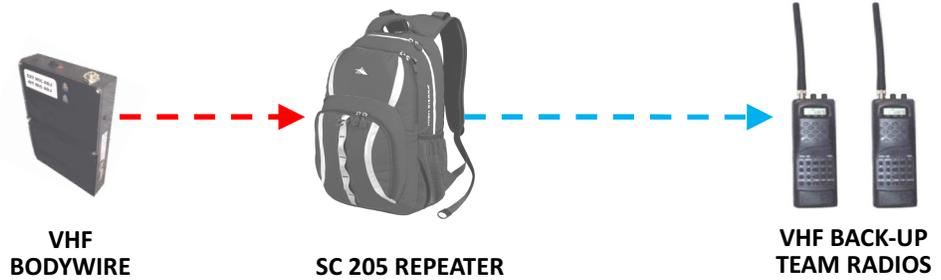
The SC 205 can transmit to P25 Public Safety secure encrypted radio communications.
