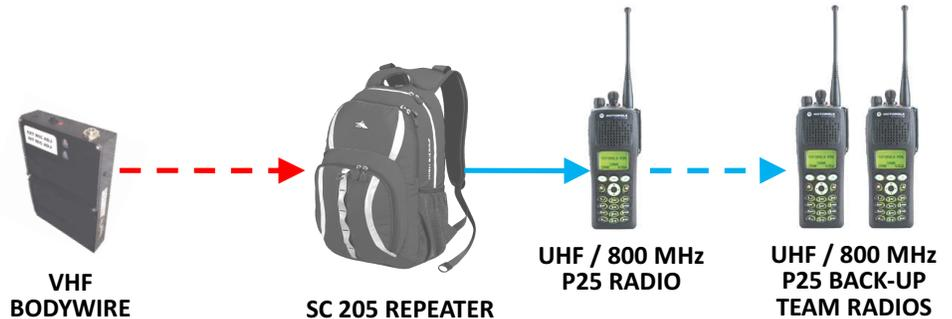
The SC 205 is designed to utilize the SpectraTek Covert Cellular Body Wire System. The SpectraTek Covert Cellular Body Wire can be used with your personal or department cell phone to integrate the audio into the repeater, transmitting to both VHF and P25 radios.
