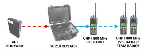
The SC 210 is designed to utilize the SpectraTek Covert Cellular Body Wire System. The SpectraTek Covert Cellular Body Wire can be used with your personal or department cell phone to integrate the audio into the repeater, transmitting to both VHF and P25 radios.
