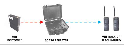
The SC 210 can transmit to P25 Public Safety secure encrypted radio communications.
